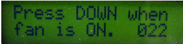
3. The Air Flow Trigger point is now set. The Air Flow Trigger is approximately half way between the Off Set Point and the On Set Point.
