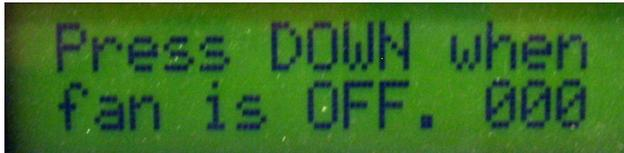
1. First turn the air mover OFF. When the fan is off and the number stops changing, press **DOWN**. This is the Off Set Point.
